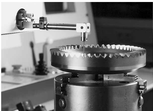
Computerized mapping of gear tooth profile
