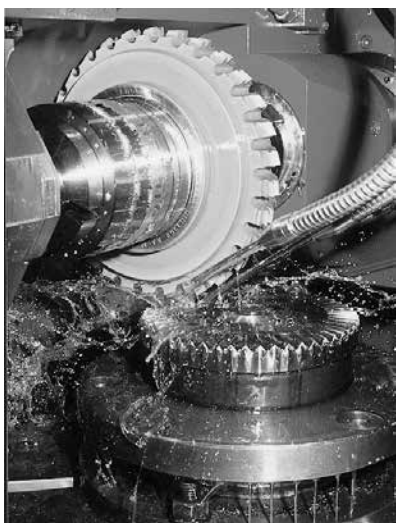
CNC machining of a PowerTRUE right-angle gear
